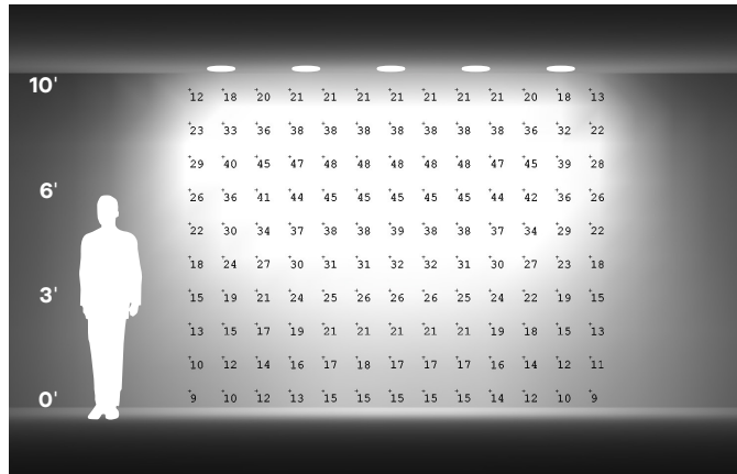
(5) SP6ES-20L35K-DX-AR6WES-MW A DISTANCE 2'6" B SPACING 2'6" O.C.
